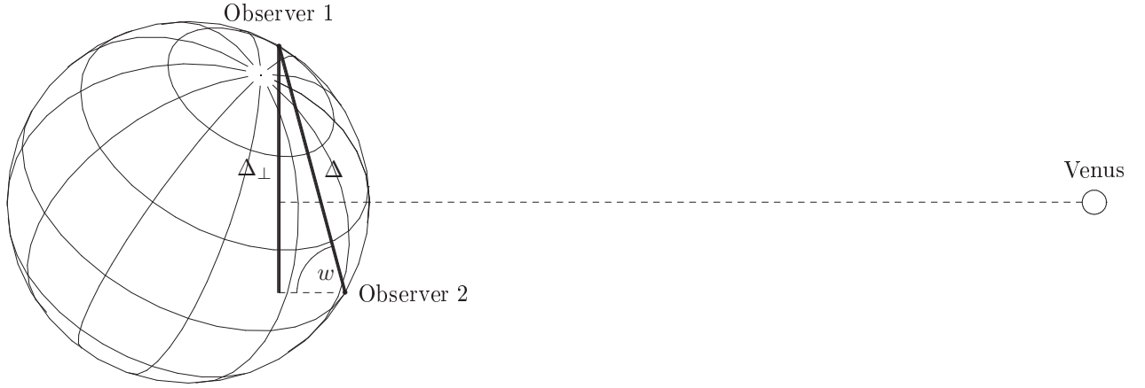
Figure 10: Not the distance \Delta between the both observers itself is important for the determination of the Sun's parallax but its projection \Delta_{\perp} parallel to the direction to Venus.
