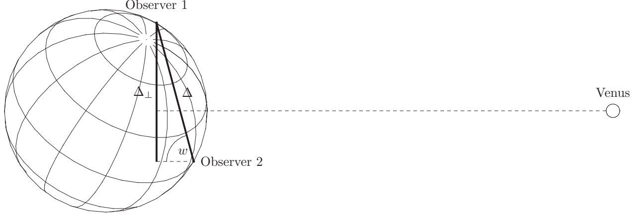
Figure 9: Not the distance \Delta between the both observers itself is important for the determination of the Sun's parallax but its projection \Delta_{\perp} parallel to the direction to Venus.
